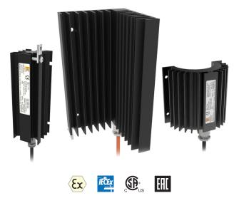
PTC heating elements produce more power when it is needed at lower temperatures. As ambient temperature increases, the resistance of the PTC element increases with the effect of a steady reduction in power output so that no power is produced above a particular temperature set point.
